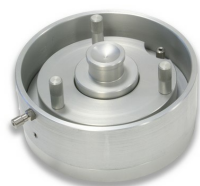
Consolidation cell, suitable for incremental loading test, swelling and permeability tests
