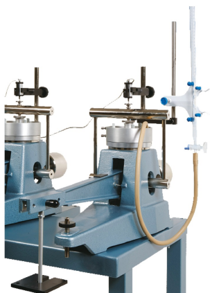
26-WF0338/A Permeability attachment fit to the 26-WF0302 with 26-WF0320 cell
