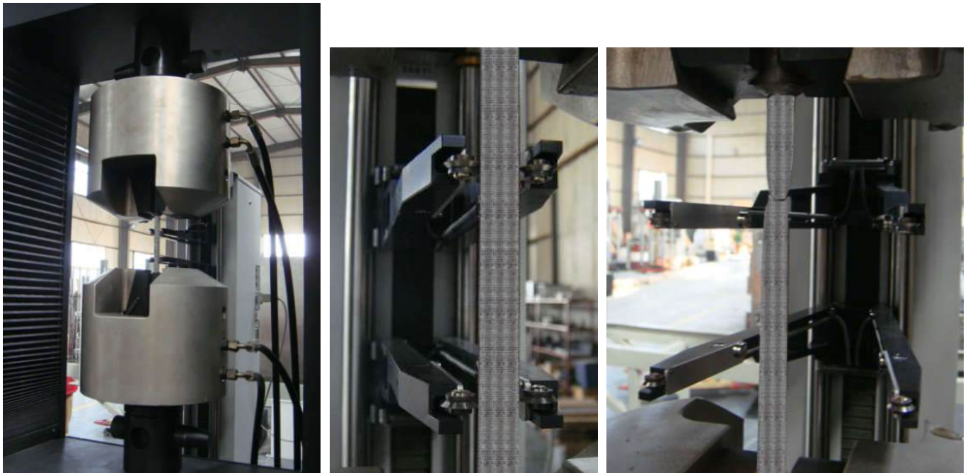
MFL with 150kN hydraulic wedge type grip
