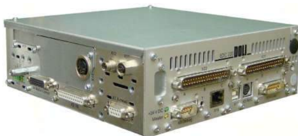
EDC 220 Intelligent Controller from Doli Germany with sampling rate 1000Hz
