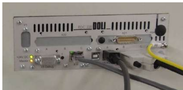
EDC 220 Intelligent Controller from Doli Germany with sampling rate 1000Hz
