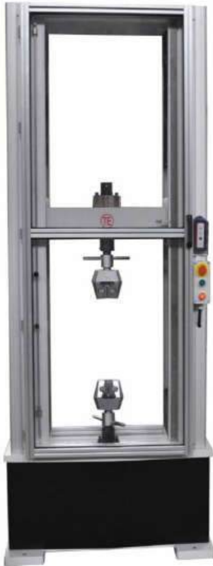
Load frame with safety shield
