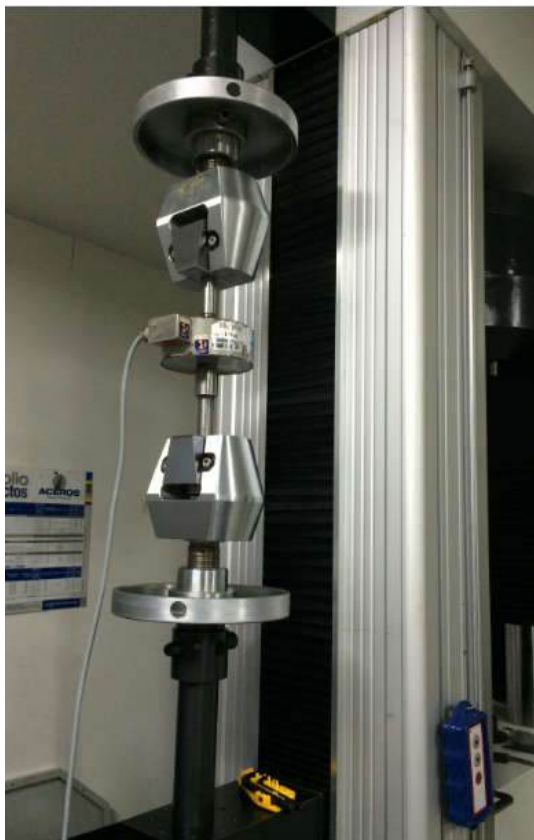
Third testing space tension calibration
