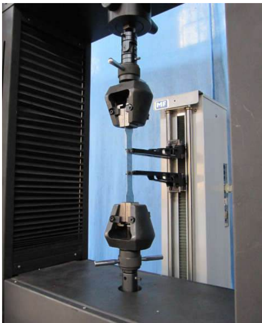
MF with 10kN Mechanical wedge type tensile grip
