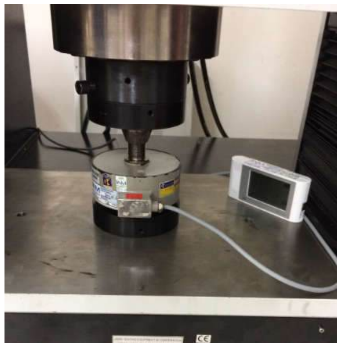
Main testing space compression calibration 60kN-600kN and 20kN-60kN
