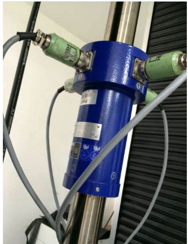
Main testing space tension calibration
