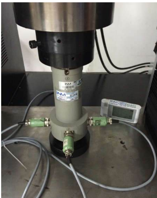
Main testing space compression calibration 60kN-600kN and 20kN-60kN
