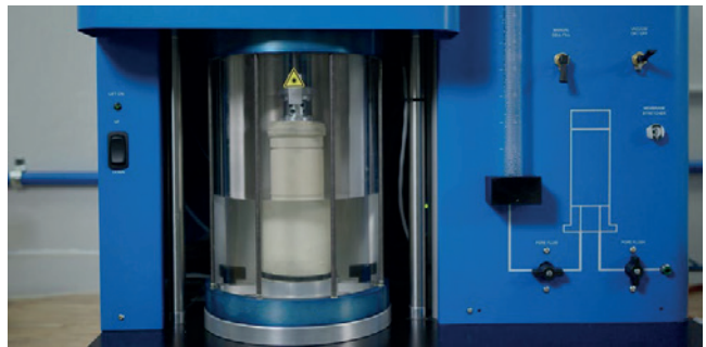
Automatic quick cell assembly and water filling/draining
