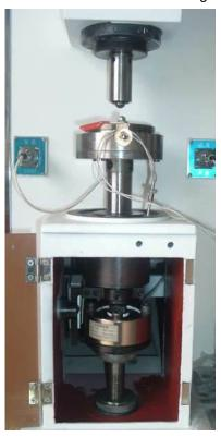
2. AC servo driving system & loading system 1 set
